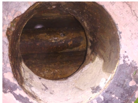
Corrosion of the boiler wall due to calcium build-up; this can reduce the efficiency of the boiler and lead to leakage of boiling water.
